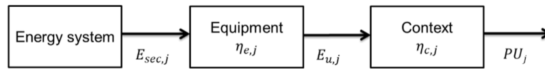
Figure 4. Extension of the energy balance for the j use: secondary energy, useful energy and provision unit.
