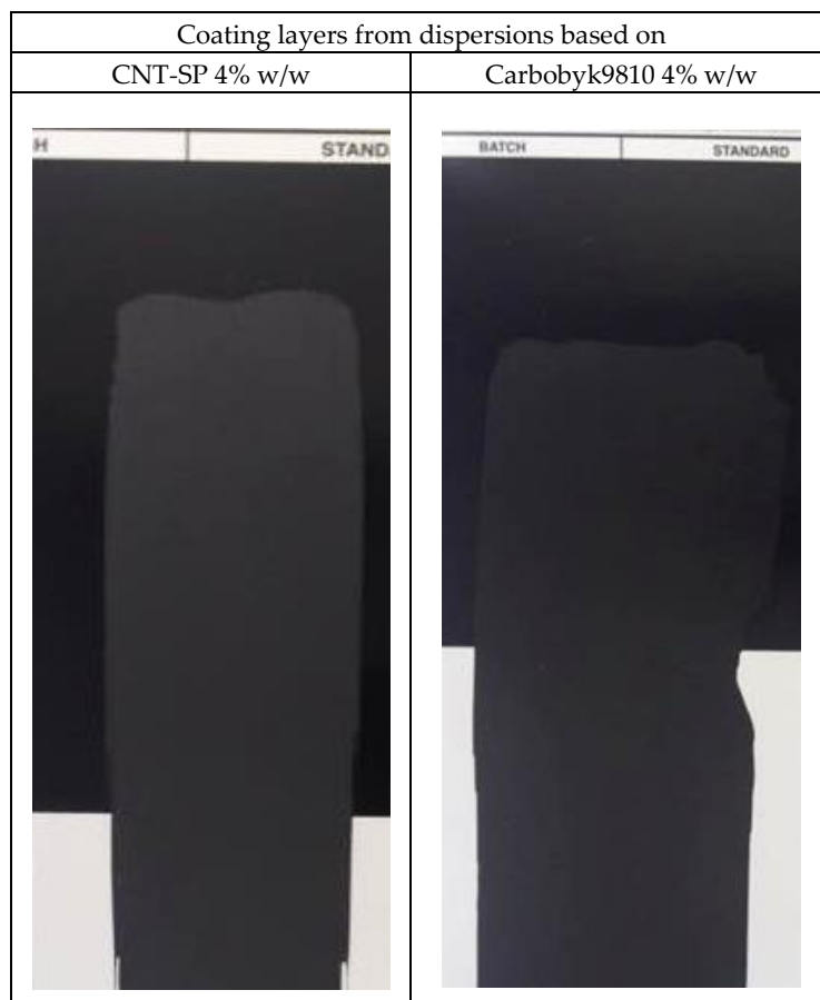
Figure S14. Coating layers from dispersions based on CNT-SP adduct (left) and on Carbobyk 9810 (right). Wet coating thickness: 100 \mu\text{m} corresponding to 20 \mu\text{m} of dried coating.
