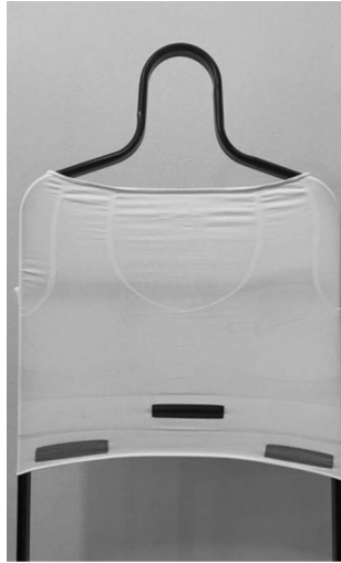
Fig. 2 - Piezoresistive sensors manufactured into flexible textile
