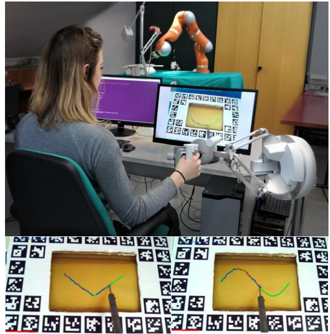
Fig. 1 The tele-operation setup comprised an LWR4+ robot and a Sigma 7 master device. To perform the task the user placed the tool on a silicone phantom and followed the path overlaid on the camera view shown on the display. The bottom images show the paths used in the test experiments (left: task 1, right: task 2).
