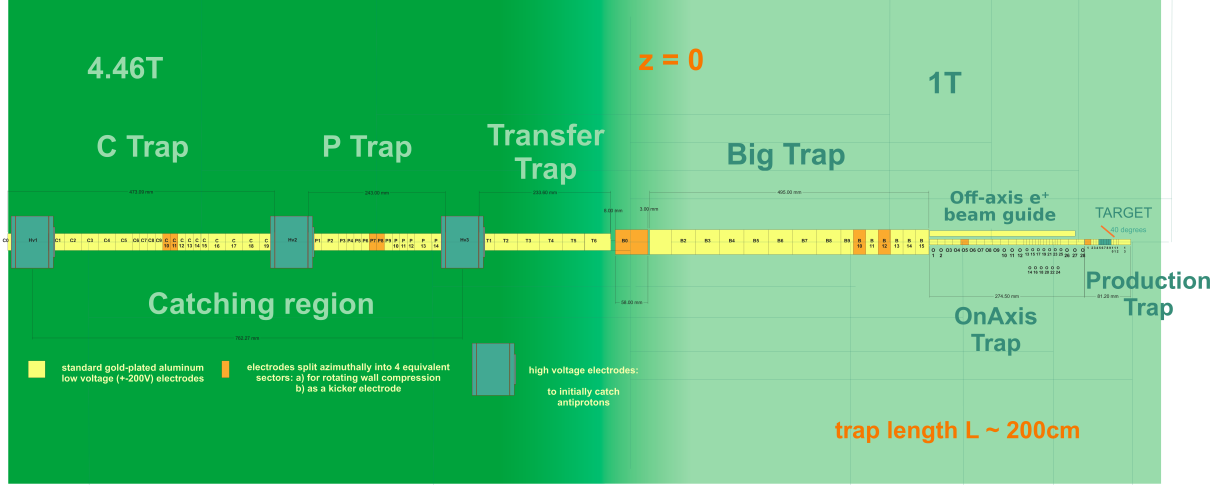
Figure 2. The main trap assembly contains a stack of \sim 190 electrodes placed in the evacuated and cryogenic core of two superconducting solenoid magnets that give rise to a homogeneous magnetic field. The Ctrap and Ptrap which are located in the 4.46 T region are used for loading electrons (Ctrap) as well as the manipulation/preparation of electron and combined electron-antiproton plasmas (Ptrap). The transfer trap bridges the crossing from the high-field 4.46 T catching region to the 1 T antihydrogen production region. The Big Trap, the OnAxis Trap and the antihydrogen production trap are located in the 1 T field. The Big Trap is important for loading electrons into the production trap while the OnAxis trap can be used for plasma oscillation studies. Positrons are injected into the positronium target located above the antihydrogen production trap through the e^+ beam guide. The production trap is designed for the purpose of pulsed antihydrogen production, cf. Fig. 4. The higher field of 4.46 T is beneficial for catching and manipulating antiprotons while the lower 1 T field prevents significant quenching and thereby loss of either Rydberg positronium or antihydrogen.
