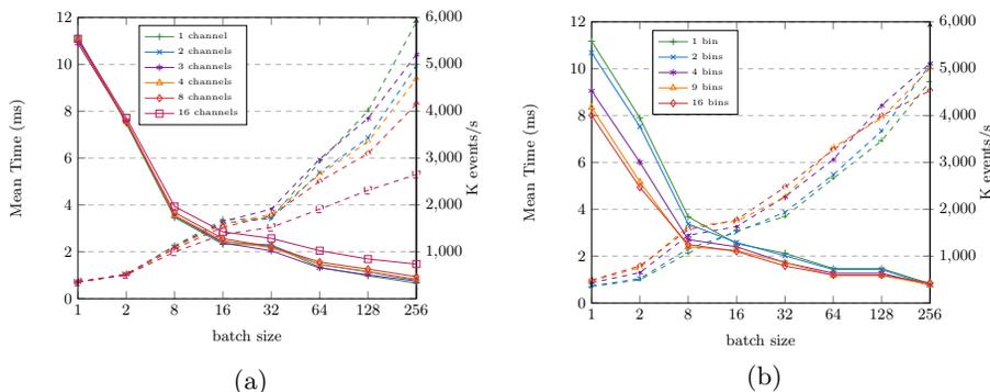
**Fig. 2.** Number of processed events per second (dashed lines) and timing (solid lines) with varying number of channels (a), and bins (b)
