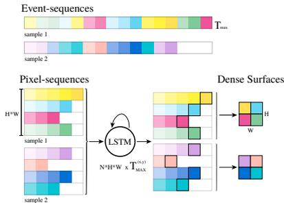
**Fig. 1.** An example of the *groupByPixel* operation on a batch of  $N = 2$  samples and a  $2 \times 2$  pixel resolution. Different colors refer to different pixel locations while intensity indicates time. For clarity, the features dimension is not shown in the figure
