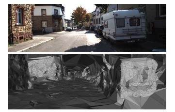
Fig. 1. Mesh reconstruction in real-time with the proposed algorithm.
