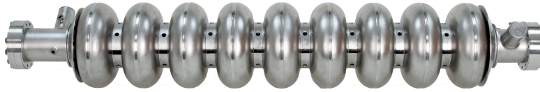
FIG. 1. A superconducting TESLA cavity. (Copyright 2006 DESY)
