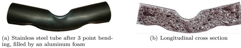
**Fig. 7** Steel tube
