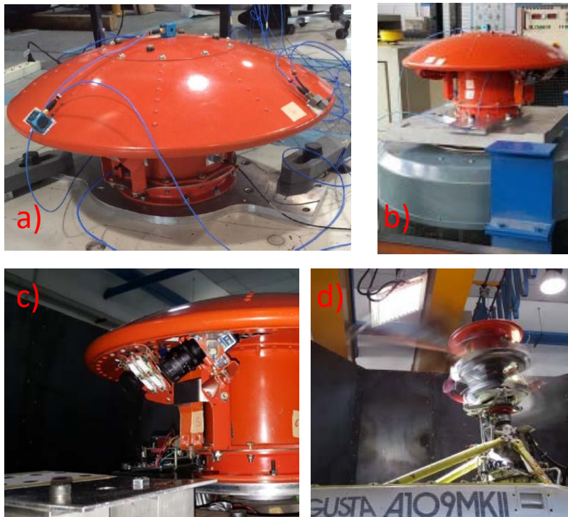
Fig 4. Harsh dynamic tests: (a) modal tests; (b) vibration tests; (c) rotation tests and sunlight sensitivity tests; (d) sunlight sensitivity tests, with the calibrated light in the upper position
