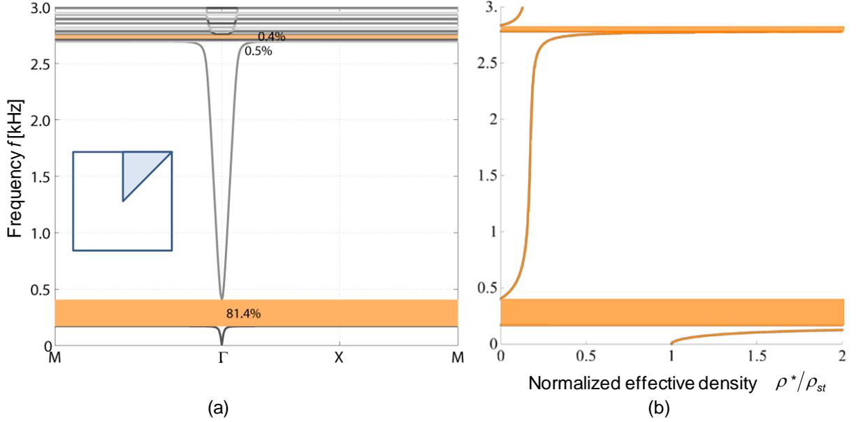
Figure 6. Three components metamaterial, filling fraction 0.4,  $R_f/R_c = 0.87$ : (a) dispersion plot with dashed bandgaps, (b) normalized effective mass density vs frequency, shaded areas correspond to negative effective mass.
