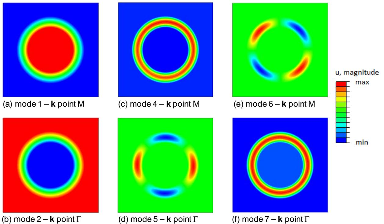
Figure 5. Three components metamaterial, filling fraction 0.4,  $R_f/R_c = 0.67$ : (a) opening mode of first band gap, (b) closing mode of first band gap, (c) opening mode of second band gap, (d-e) flat modes inside second band gap, (f) closing mode of second band gap.
