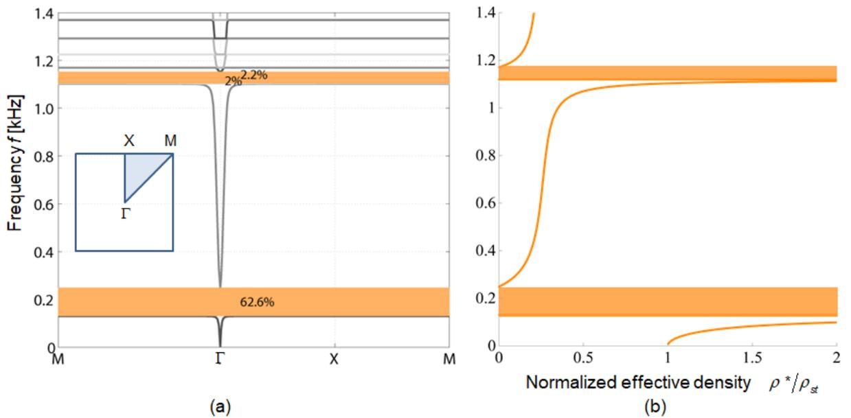
Figure 4. Three components metamaterial, filling fraction 0.4,  $R_f/R_c = 0.67$ : (a) dispersion plot with dashed bandgaps, (b) normalized effective mass density vs frequency, shaded areas correspond to negative effective mass.
