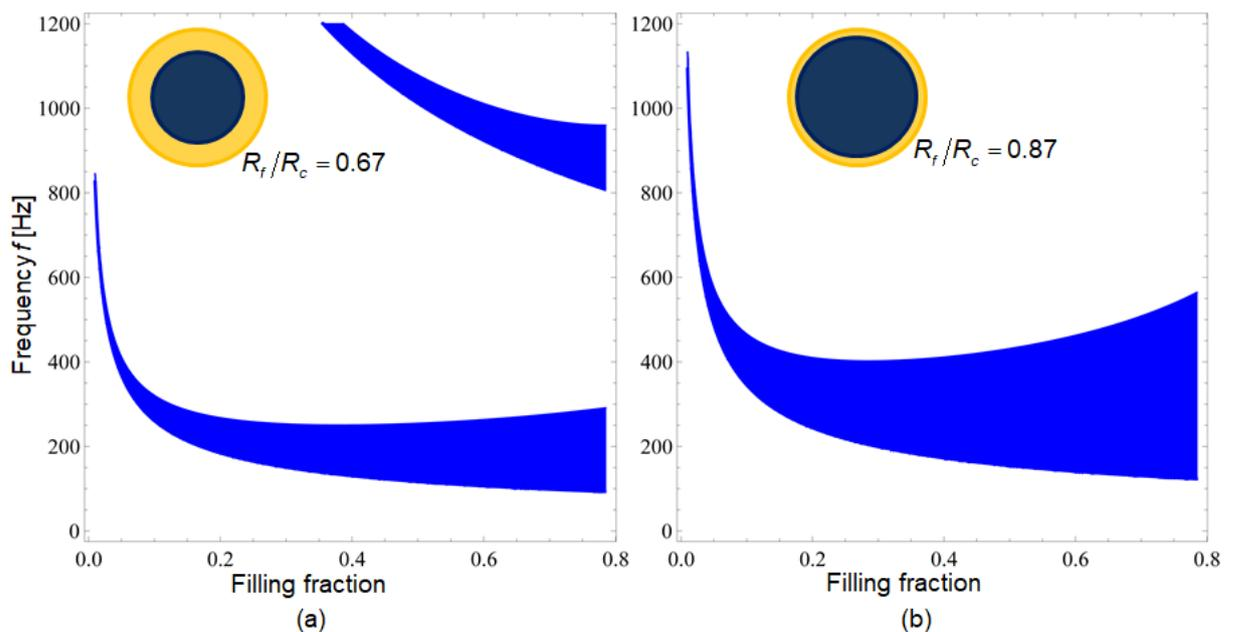
Figure 3. Frequency intervals of negative effective mass for varying filling fraction: (a) thick coating  $R_f/R_c = 0.67$ , (b) thin coating  $R_f/R_c = 0.87$ .
