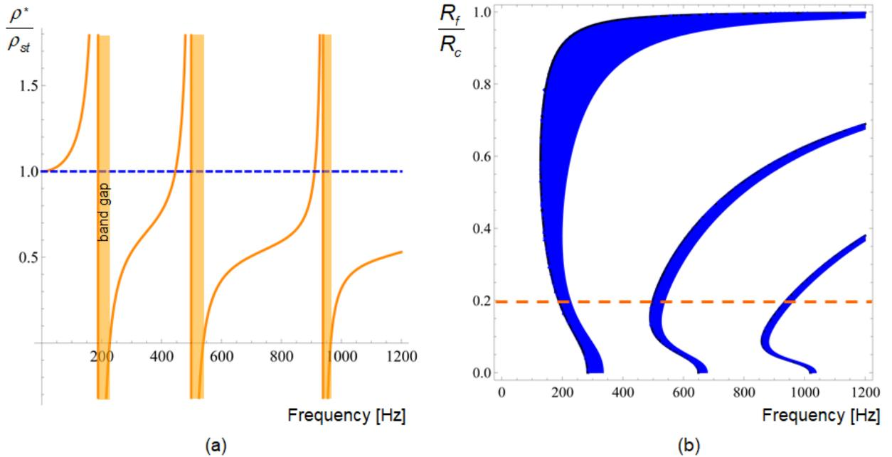
Figure 2. Ternary metamaterial with filling fraction 0.4: (a) normalized effective mass vs. frequency for  $R_f/R_c = 0.2$ , intervals of negative effective mass give the first three band gaps; (b) intervals of negative effective mass in the plane frequency-  $R_f/R_c$ , the dashed line corresponds to the case shown on the left.
