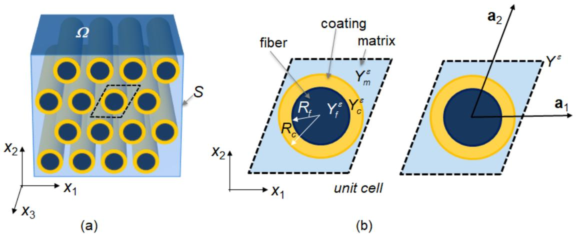
Figure 1. Metamaterial with periodically distributed coated cylindrical inclusions: (a) geometry, (b) unit cell with primitive vectors  $\mathbf{a}_i$ .
