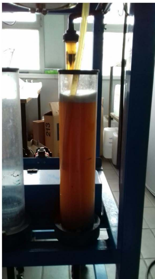
Figure S1: Picture of the non-treated real pharmaceutical IWW with the strong dark orange colorization.
