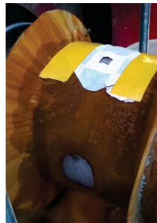
Figure 6: Details of the corrosion fatigue experiments: a) The adopted full scale specimen with EDM notches; b) test bench with the dropping system; c) detailed observations on 10 \text{ mm}^2 areas.
