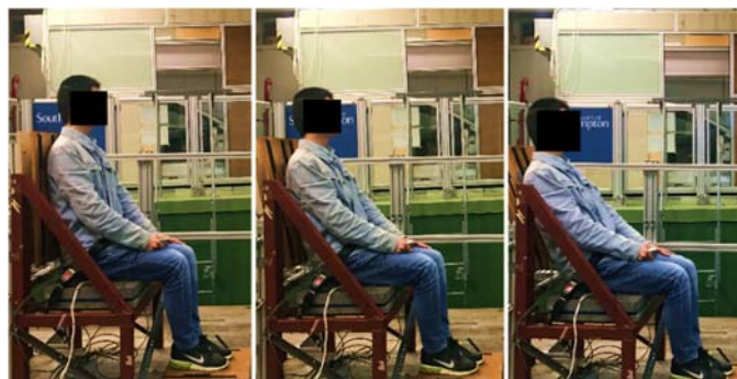
Figure 2: The postures of the subject sitting in the seat with different angles of backrest inclination (from left to right: 0^\circ , 10^\circ , and 20^\circ )
