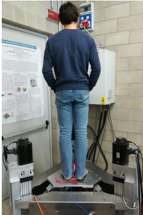
Figure 2: Subject standing on the sensorized insoles, without shoes on the three-axis shaker, shown with the reference system used.
