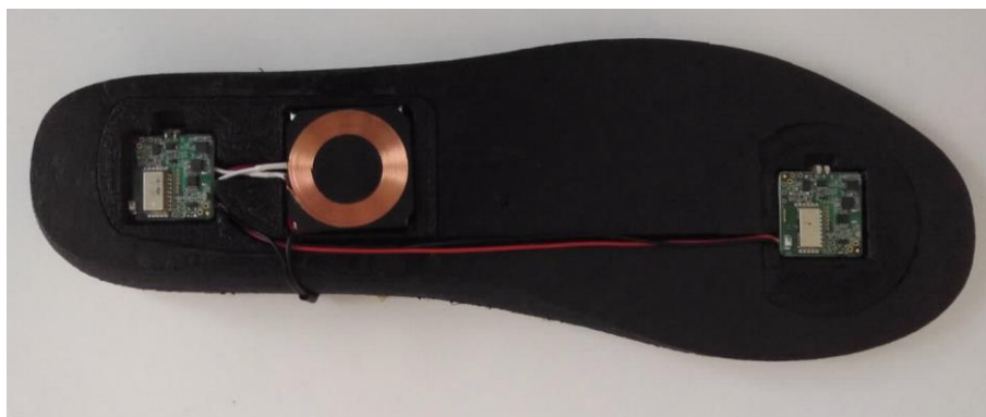
Figure 1: Photograph of the data acquisition and transmission system inside the insole
