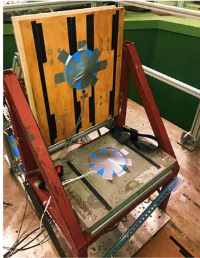
Figure 1: The rigid seat, rigid backrest, force plate at the seat pan, force transducers at the backrest (only the screws securing the transducers are shown) and SIT-pads used in the experiment
