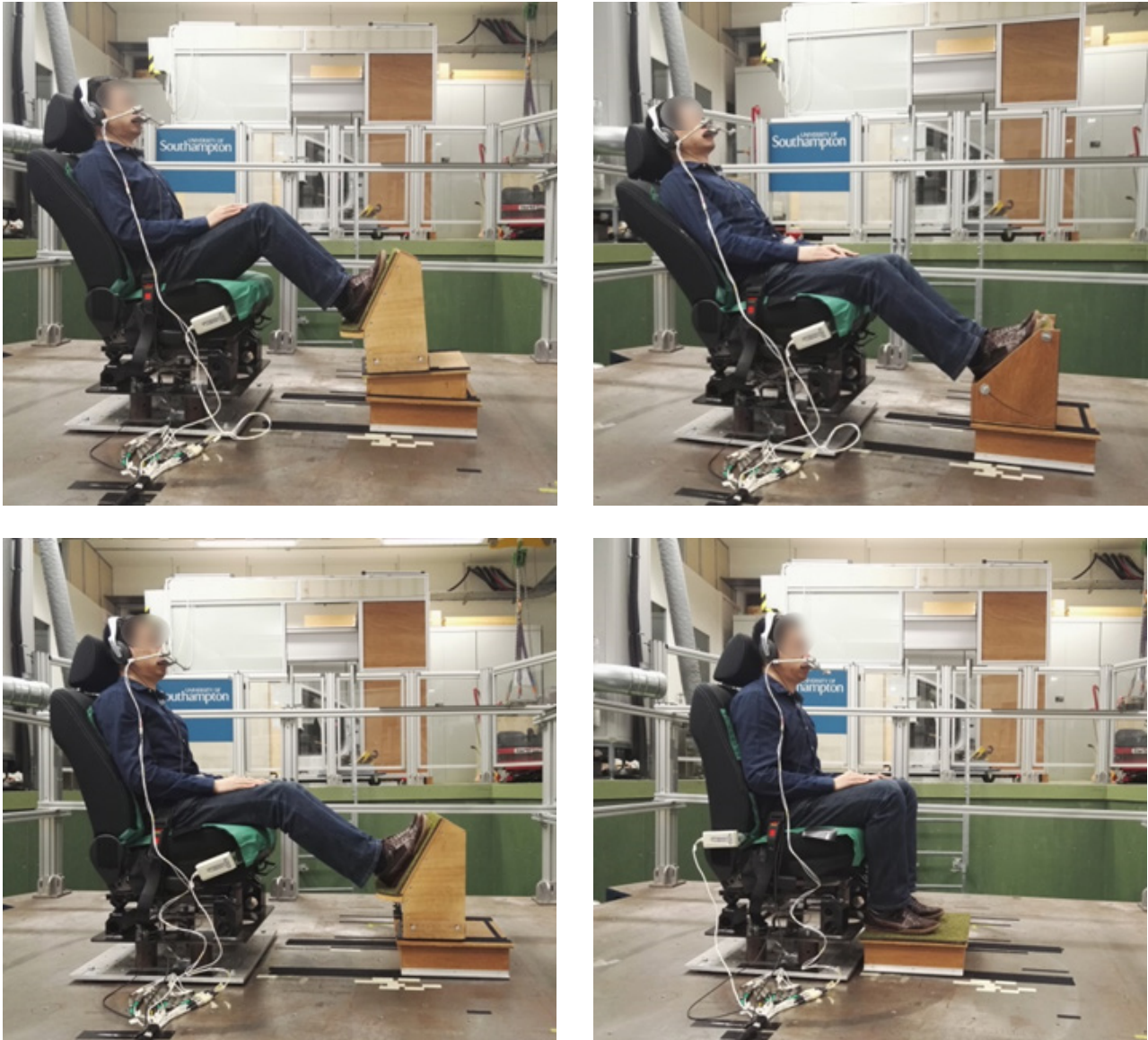
Figure 1 Sitting configurations. Top left: ( self- ) entertaining/socialising (ES). Top right: relaxing/sleeping (RS). Bottom left: travelling/driving (TD). Bottom right: working/eating (WE).
