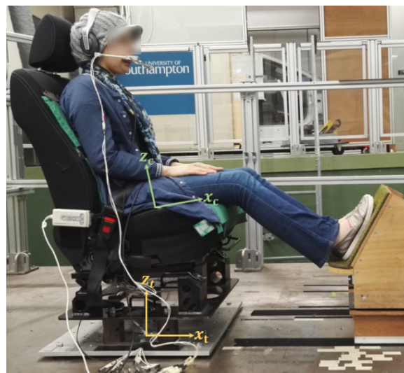
Figure 2 Experimental arrangement and coordinate systems. \{x_t, y_t, z_t\} : coordinate system at vibration table. \{x_c, y_c, z_c\} : coordinate system at interface between seat cushion and occupant buttocks.
