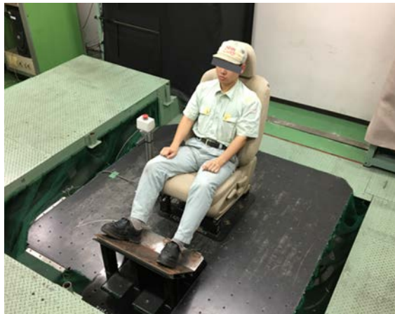
Figure 8: Laboratory apparatus for lateral human body shaking evaluation
