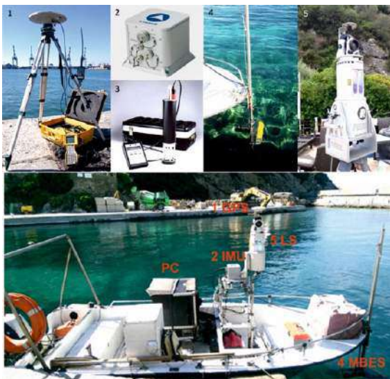
Figure 2. On board technical equipment for the integrated survey: 1) GPS-RTK; 2) IMU; 3) SVP; 4) MBES; 5) LS.
