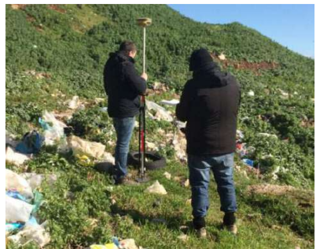
Figure 7. GNSS survey of the aluminium targets.
