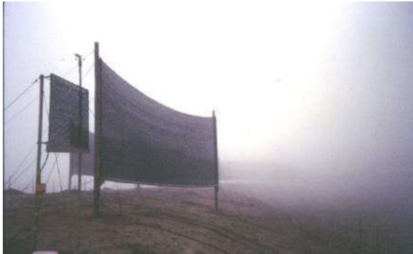
Figure 1. A Standard Fog Collector and a Large one in the Lomas the Mejia
