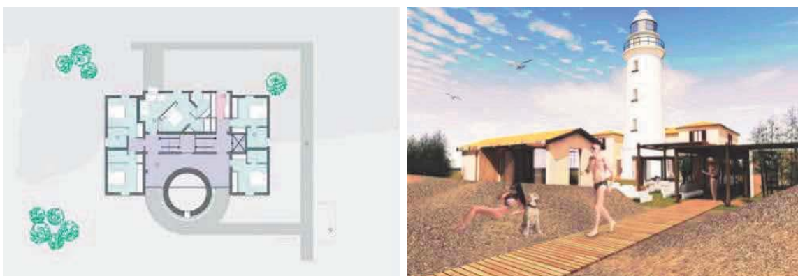
Fig. 05/06 : Goro Lighthouse: reuse general plan, first floor. Right: a project rendering: the lighthouse with the proposed removable wooden structure as seen from the seaside
