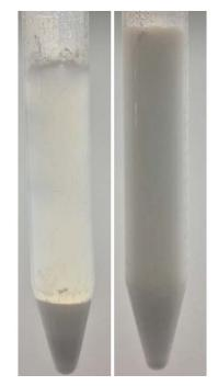
**Figure 6.** Powders *i* (left) and *d* (**right**) redispersed after spray drying.
