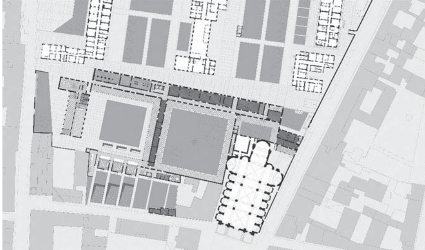
Fig. 5 Ground floor plan. Project of the completion of the cloister with limited volumetric increments
