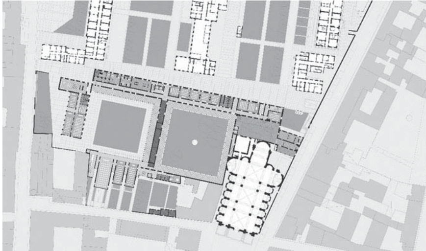
Fig. 7 Ground floor plan. Project of the completion of the cloister with maximum volumetric increment
