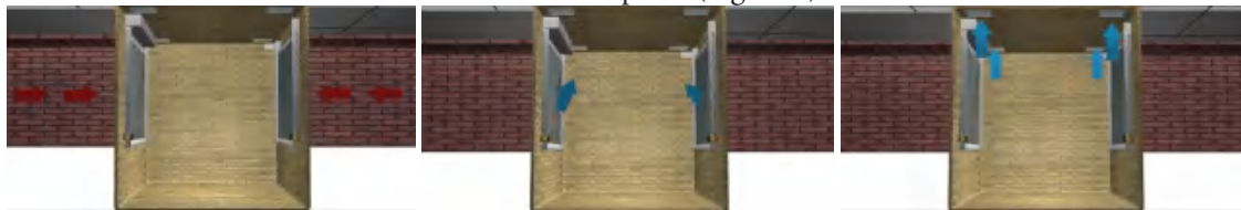
[Figure 2] Air flow through the windows composed by three cellulose pads in the technical room placed at the basement of the building.
