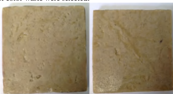
[Figure 5] Samples of recycled PLA with addition of jute fiber both sides.
