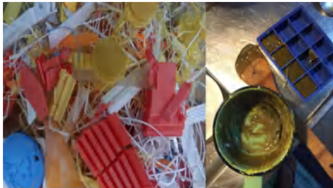
[Figure 2] PLA wastes used in this work (left), enameled pan and silicone mold (right).
