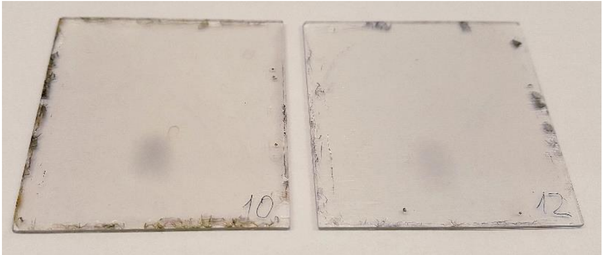
Fig. S1. Picture of two emulsion detectors after exposure to the beam and chemical development. (Photo credit: Ciro Pistillo , Università degli Studi di Milano).
