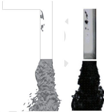
Figure 21: Internal nozzle flow test case [52]. Left) interPhaseChangeMixingFoam ; right) visualizations from experiments.
