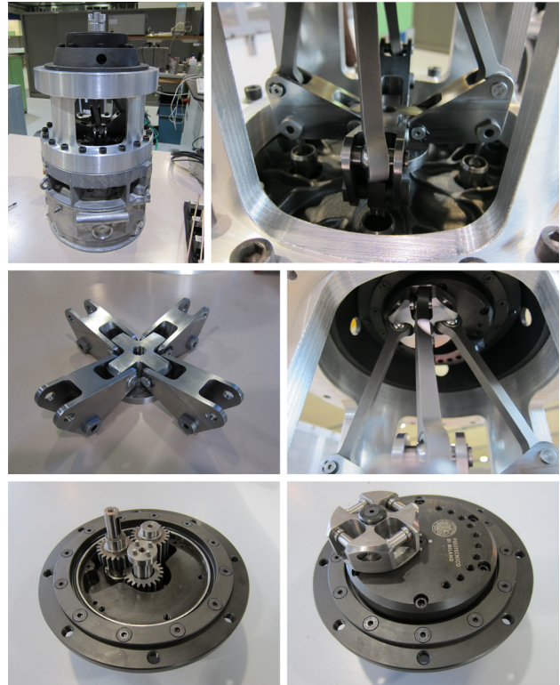
Fig. 9 Pictures of the mechanical components of the proposed kinematic scheme for a four-cylinder configuration
