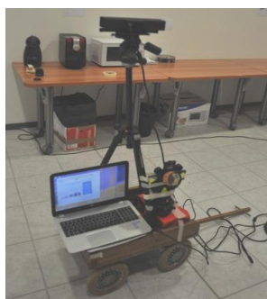
Figure 5. The Kinect installed together with the laptop and the reflective prism on the cart
