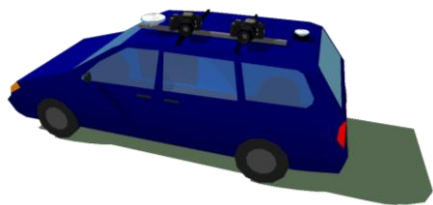
Figure 1. Scheme of the vehicle equipped with two cameras and two GPS antennas used for the kinematic tests
