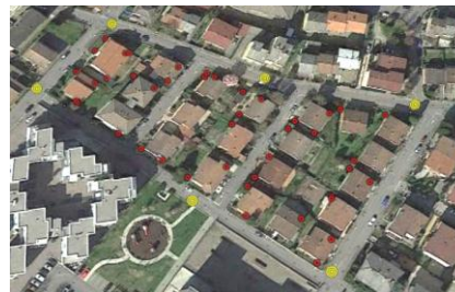
Figure 2. The residential area selected for the kinematic test. The selected GCPs are represented in red, while the GPS pseudo-observations in yellow.
