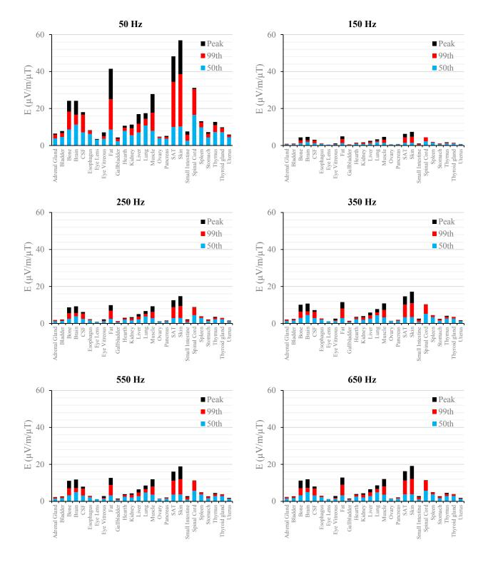
**Figure 6.** E ( $\mu$ V/m) per  $\mu$ T of 50 Hz B<sub>peak</sub> induced in foetal tissues at 9 mGA for all the harmonic frequencies considering the standard EN 50160 for the LV&MV power supply networks. The bars indicate the E<sub>50th</sub> (blue), the E<sub>99th</sub> (red) percentiles and the E<sub>peak</sub> (black) of each distribution.
