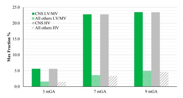
**Figure 9.** Maximum fraction of the ICNIRP Basic Restrictions for general public on the E<sub>99th</sub> for the CNS and all other tissues, exposed to a magnetic field at the reference level using the standard EN 50160 (B levels shown in Table 4), at different GA.
