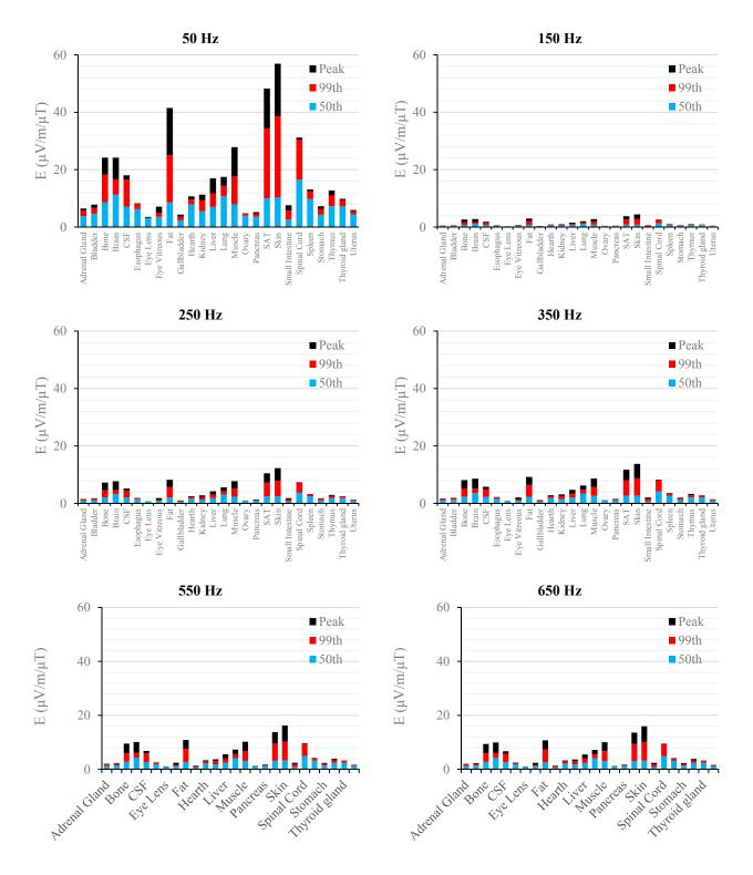
**Figure 7.** E ( $\mu$ V/m) per  $\mu$ T of 50 Hz B<sub>peak</sub> induced in foetal tissues at 9 mGA for all the harmonic frequencies considering the standard EN 50160 for the HV power supply networks. The bars indicate the E<sub>50th</sub> (blue), the E<sub>99th</sub> (red) percentiles and the E<sub>peak</sub> (black) of each distribution.
