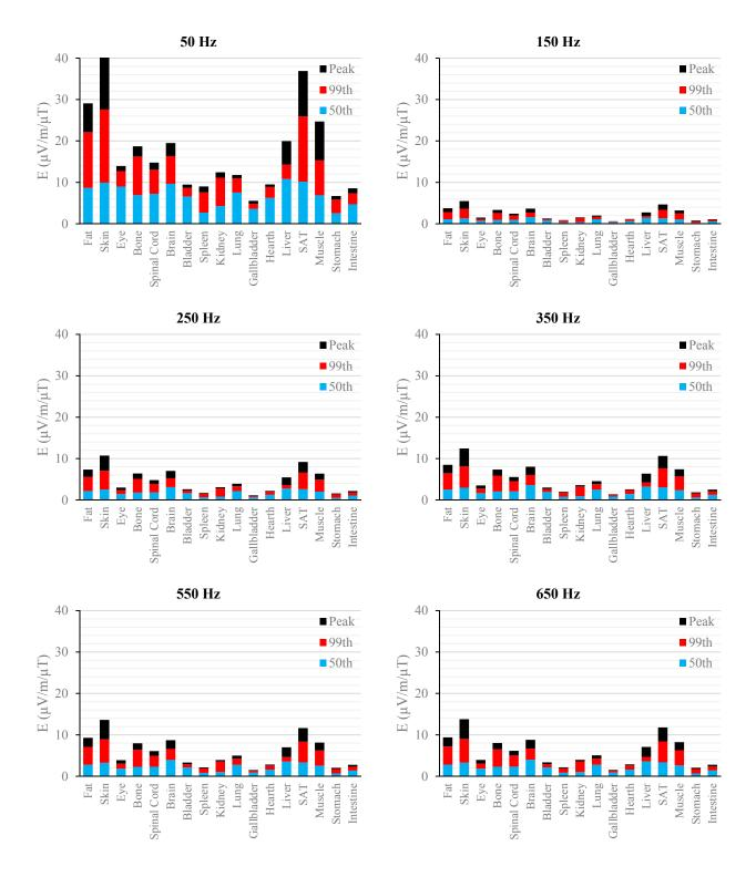
**Figure 4.** E ( $\mu$ V/m) per  $\mu$ T of 50 Hz B<sub>peak</sub> induced in foetal tissues at 7 mGA for all the harmonic frequencies considering the standard EN 50160 for the LV&MV power supply networks. The bars indicate the E<sub>50th</sub> (blue), the E<sub>99th</sub> (red) percentiles and the E<sub>peak</sub> (black) of each distribution.
