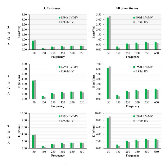
**Figure 8.** E<sub>99th</sub> (mV/m) induced over CNS tissues (left) and all other tissues (right) at different GA as a function of the frequency of the component under investigation for the worst-case exposure (see the text for details). The green and grey bars indicate the two classes of networks identified by the EN 50160 standard, *i.e.*, Low and Medium Voltage (LV & MV) and the High Voltage (HV) networks, respectively.
