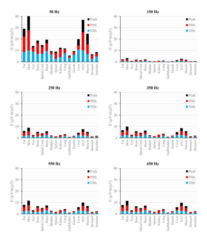
**Figure 5.** E ( $\mu$ V/m) per  $\mu$ T of 50 Hz B<sub>peak</sub> induced in foetal tissues at 7 mGA for all the harmonic frequencies considering the standard EN 50160 for the HV power supply networks. The bars indicate the E<sub>50th</sub> (blue), the E<sub>99th</sub> (red) percentiles and the E<sub>peak</sub> (black) of each distribution.
