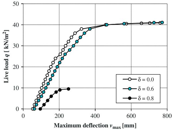
Figure 17. Arch bridge: load versus maximum deflection of the central main beam of the deck for the cases of undamaged bridge ( $\delta = 0$ ) and bridge with damaged suspension steel ties with corrosion penetration depth  $\delta = 0.6$  and  $\delta = 0.8$ .
