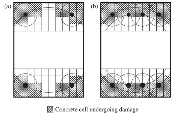
Figure 2. Definition of the zones of concrete cover undergoing damage: mechanism of cover spalling with (a) inclined fracture planes for wide bar spacing, and (b) parallel fracture planes (delamination) for closely spaced bars.
