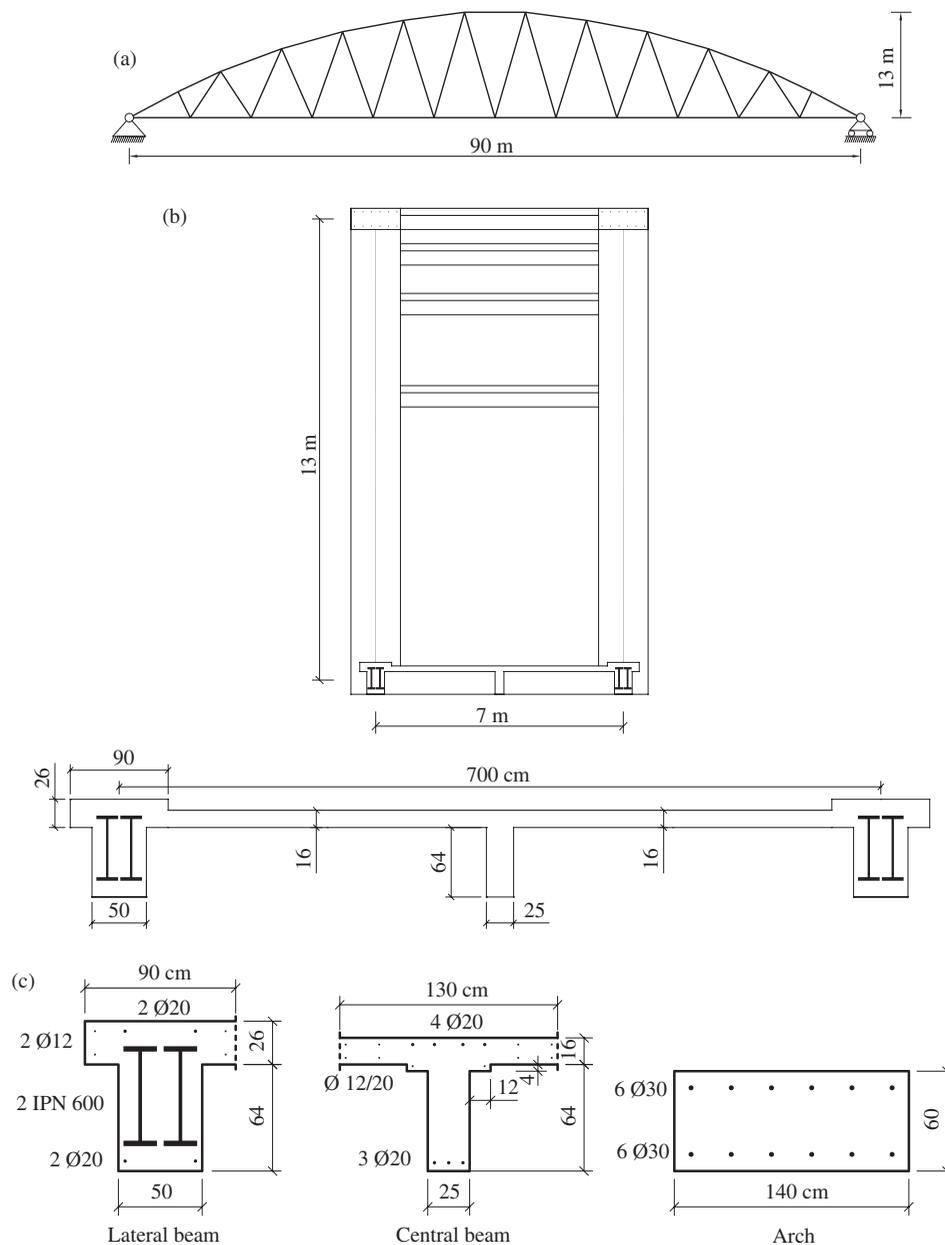
Figure 12. RC arch bridge exposed to corrosion: (a) structural scheme, (b) cross-section view of bridge deck and arches, and (c) cross-sections of the deck's main beams and of the arches.
