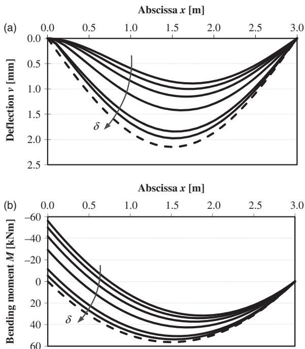
Figure 10. Statically indeterminate beam: (a) deformed shape and (b) bending moment diagram for different values of corrosion penetration depth ( $\delta = 0, 0.2, 0.4, 0.6, 0.8, 1.0$ ), compared with the limit case of undamaged simply supported beam (dashed curve).
