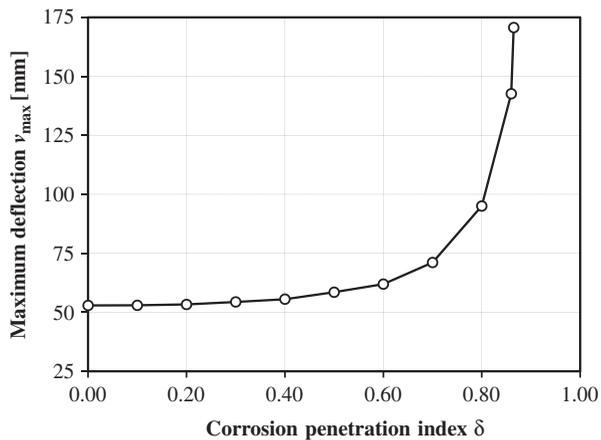
Figure 18. Arch bridge: maximum deflection of the central main beam of the deck under dead load ( $q = 0$ ) versus the corrosion penetration index for the case of bridge with damaged suspension steel ties.
