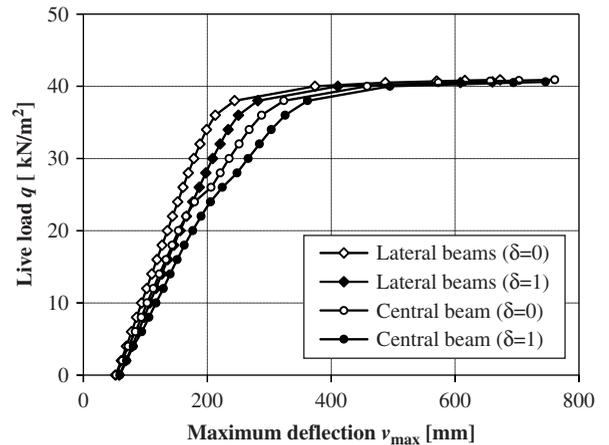
Figure 16. Arch bridge: load versus maximum deflection of the lateral and central main beams of the deck for the cases of undamaged bridge ( $\delta = 0$ ) and bridge with damaged arches with complete corrosion penetration ( $\delta = 1$ ).
