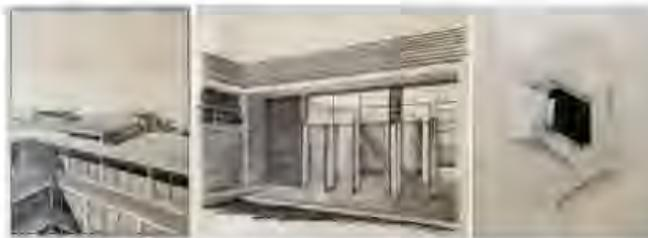
to the exterior of the building. The module of 4.50 meters that manages the building in plan is explained, unlike the previous version, outside on the fronts, thanks to the structural mesh in reinforced concrete that alternates with the closing modules (fig. 7).
