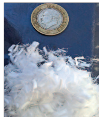
6A, 6B e 6C. Additivo super-fluidificante (6A), additivo aerante (6B) e fibre in polipropilene (6C)
