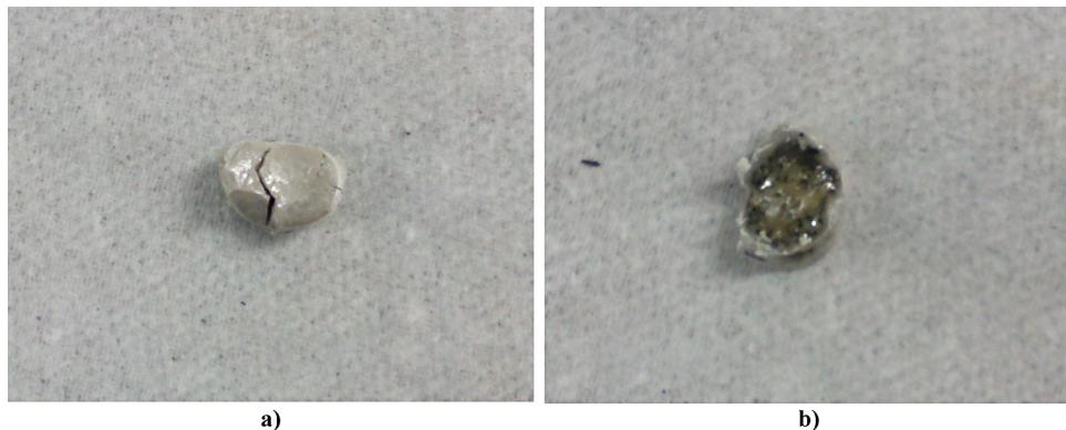
Fig. 8. Photos of CaO samples laser melted and refrozen in air (a) and in Ar + 6% H<sub>2</sub> (b).
