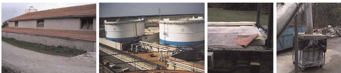
Figure 1 | Examples of diffuse sources (from left to right): unventilated livestock shed, floating-roof oil storage tanks, partially covered wastewater treatment tank and sludge storage container.
