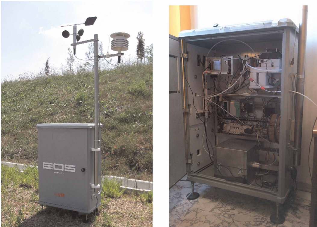
Figure 4 | The electronic nose developed by Politecnico di Milano and Sacmi s.c., in the field (left) and in the laboratory (right).
