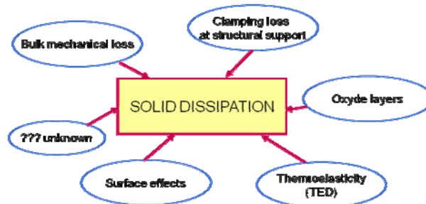
Fig. 10. Schematic representation of possible solid damping mechanisms in MEMS
