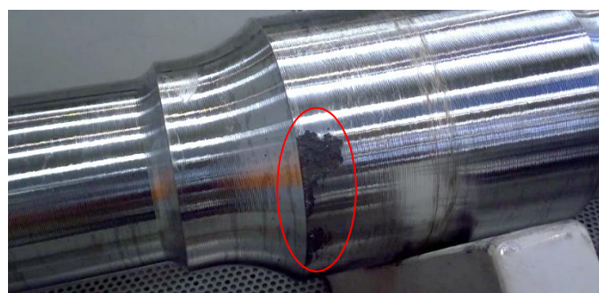
Fig. 4. Identification of missing material in a late process step.
