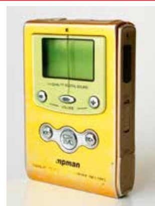
1998 Esce sul mercato MPMan, il primo lettore Mp3. Ha 32 Mb di memoria/ The MPMan music player debuted with 32 megabytes of memory. The music needed to be encoded in the MP3 format in order to play
