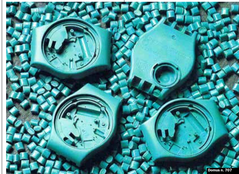
1989 Casse del modello Swatch da donna con i grani di materia plastica grezza/ Cases of the women's wristwatch by Swatch, showing granules of unmelted plastic
