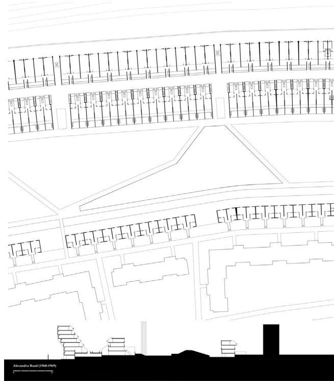
Figure 15 Alexandra Road by Neave Brown (Camden, 1967-1980). Ground floor plan and section. Source: drawing by Gerardo Semprebbon, in cooperation with D. Fusari, M. Ignaccolo, M. Mikaelyan.
