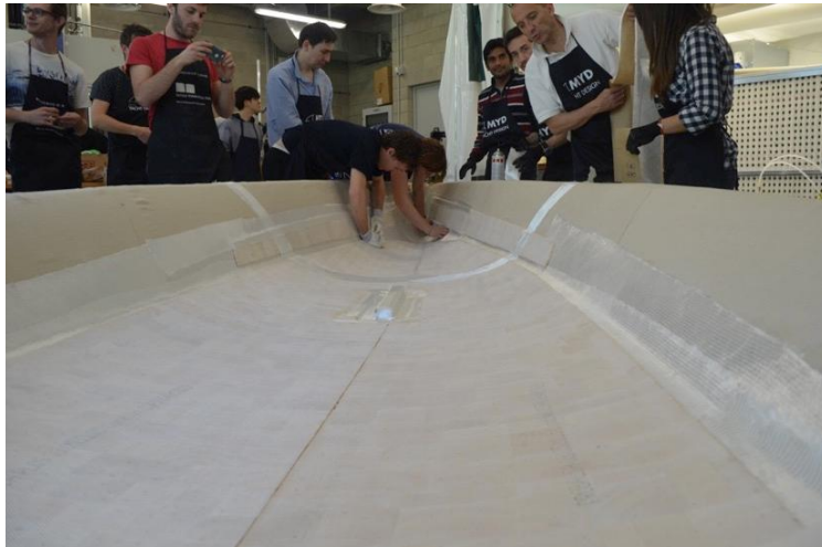
Fig.5: Hull reinforcement fibers and core placement in the female mold
