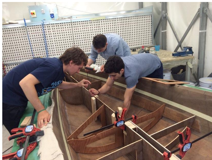
Fig.7: wooden structures in place before their lamination
