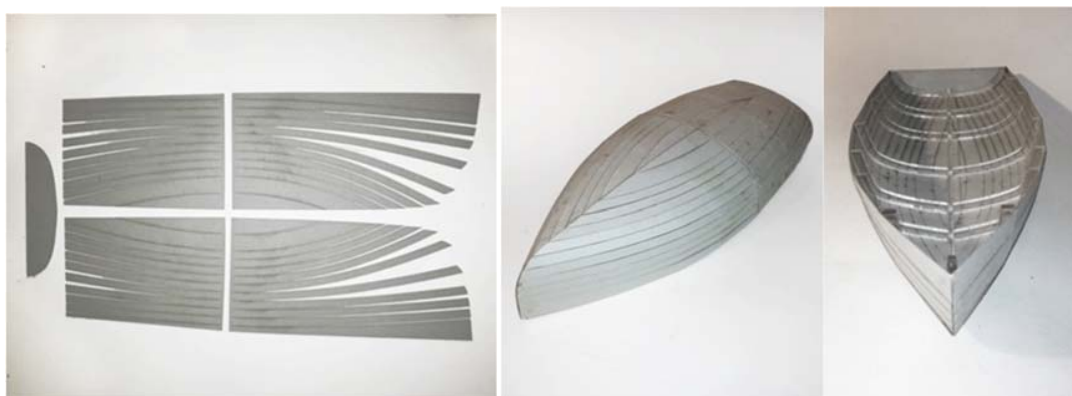
Fig. 2: Model study carried out starting from cardboard sheets
