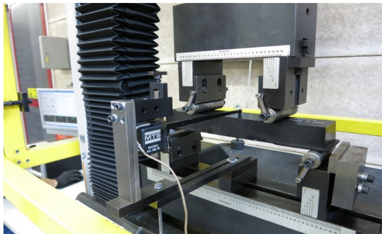
Fig. 5: Four-point bending setup
