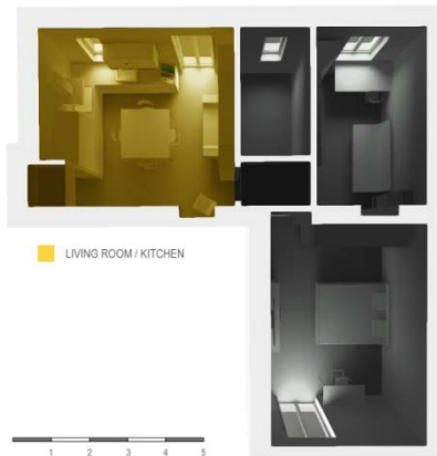
Figure 1 – Evaluated areas for the natural lighting simulation in order to access the non-visual effects of lighting on young and elderly people
