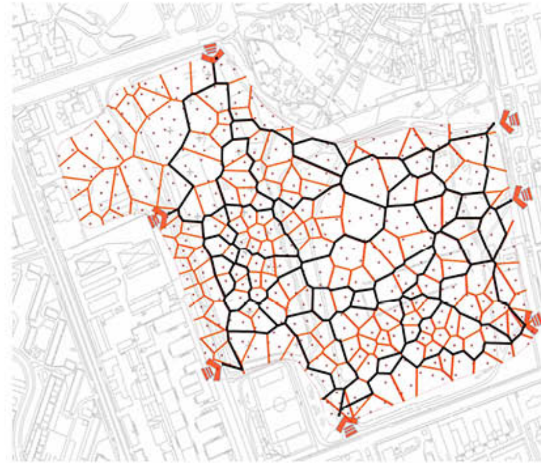
Tessellation Circulation patterns simulated by an algorithm using entry points and land features as attractors.
