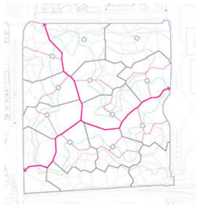
Parcels and Paths The site is subdivided by a tessellation logic that interpolates data points pertaining to water management in the area, under normal conditions as well as with exceptional rainfall levels.
