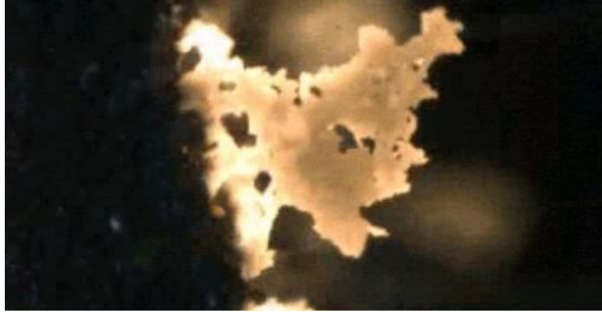
Figure 1. CCP leaving the burning surface of a nAl-based propellant (courtesy of Galfetti et al. 27 )
