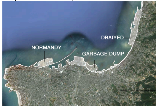
Figure 3. Beirut: landfill Normandy, is a large strip of land, about 180 hect formed, in part during the years of civil war(1975-1994),by deposit, in the sea, of waste, and in part, in a post-war time, by debris of destroyed city and even by a reconstruction plan very "intence
