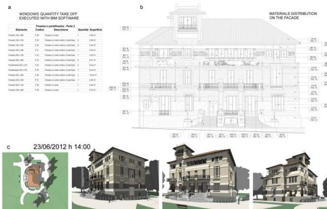
Fig. 4 Building Information Modelling for heritage buildings (Villa Faccanoni) applied in the 3D modelling course: (a) quantity take off, (b) façade material survey, (c) images from the solar analysis
