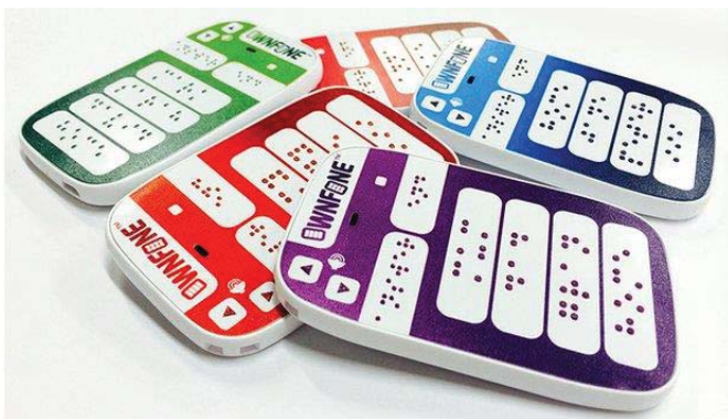
Fig. 4: OwnFone prototypes. Now in production, you personalize the haptic display with the contacts you want
