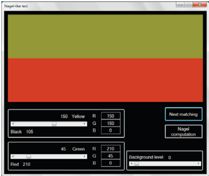
Fig. 7 - Nagel like anomaloscope. A yellow color is at the top while below is a mixture of red and green matching the yellow for a deuteranope.
