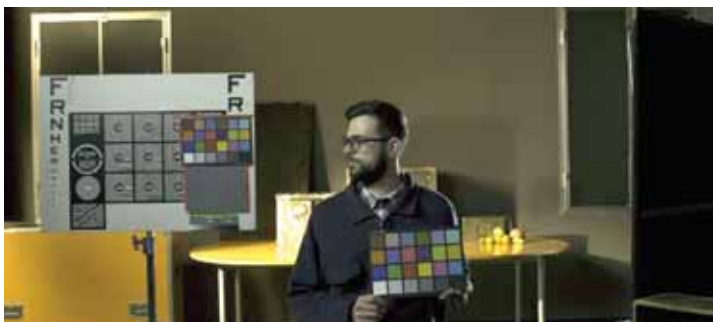
Fig. 4 – Footage from Fig.3's set (Sony F55 camera), after applying the Input Transform and an LMT into ACEScc colour space for the purpose of colour grading (washed out look is due to the tone-curve behaviour of the RRT).
