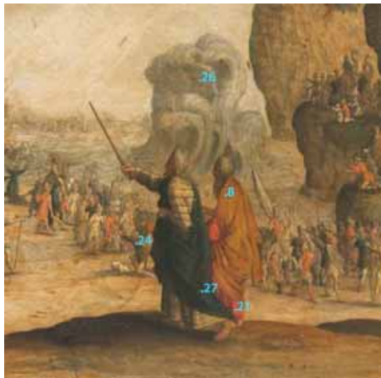
Fig. 2 – Area of the painting (DETAIL n.1) of 10 cm x 10 cm acquired by the hyperspectral imager; numbers on picture refer to the FORS analyses' measurement points.
