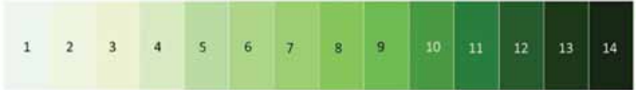
Fig. 5 – Algae colour identification scale, indicating the algae density and ranging from very light shades in transparent container to dark ones with increasing opacity. © 2013 Robert Bair, University of South Florida, https://www.teachengineering.org/view_activity.php?url=collection/usf_/activities/usf_biorecycling/usf_biorecycling_lesson01_activity2.xml
