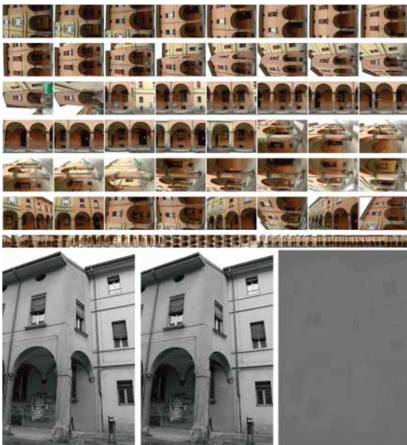
Fig. 2 - BID technique processing and results: top original dataset; middle: the mosaic of all the images; bottom left: image converted using MATLAB RGB2Gray; bottom middle: image converted via BID ; bottom right: pixel-by-pixel differences between the two images converted with RGB2Gray and BID .
