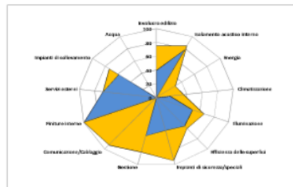
Figure 3: Esempio di report grafico delle prestazioni dell'edificio (Torre Velasca): "AS IS - TO BE" - BRaVe Office Building. Figure 3: Example of graphical report building performance (Torre Velasca): "AS IS - TO BE" - BRaVe Office Building.
