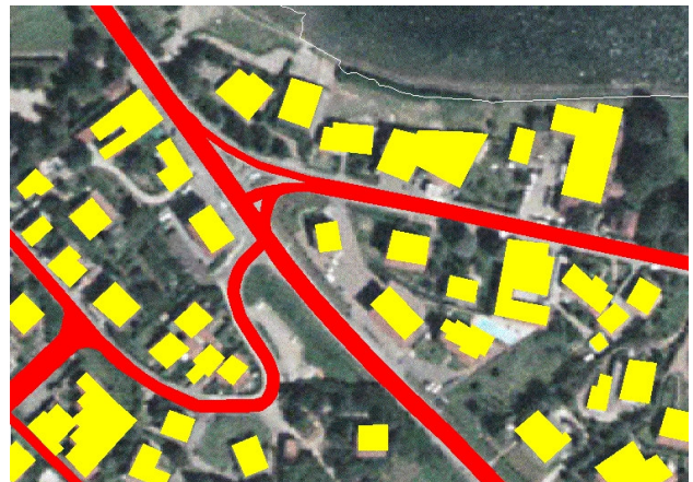
Figure 6 – Orthophotomap (1:10,000 scale) derived from aerial photogrammetry with superimposed vector layers extracted from IKONOS orthoimage.
