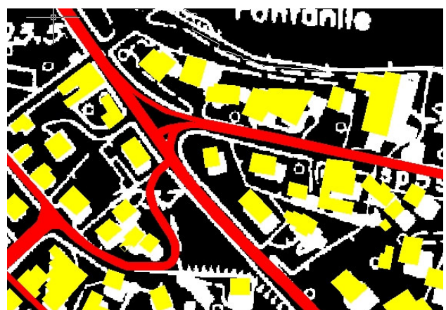
Figure 7 – Raster regional map (CTR at 1:10,000 scale) with superimposed vector layers extracted from IKONOS orthoimage.
