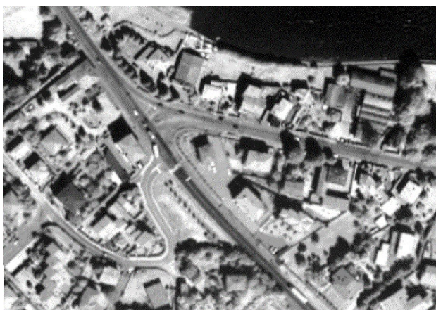
Figure 4 – Patch of the orthoimage derived from an IKONOS over the area of Lecco used in the test for evaluating the possibility for information capture from HRSI.
