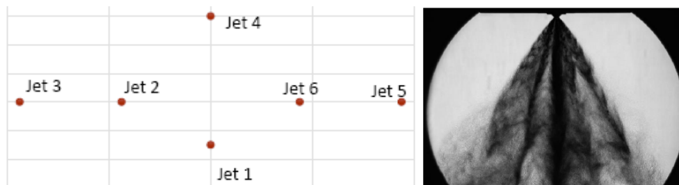
Figure 2. The spray pattern on a plane perpendicular to its axis
