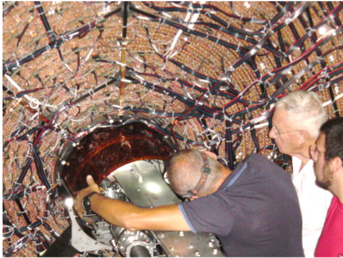
Figure 1. The insertion of the graphite target used by AMADEUS in the 2012 run inside of KLOE setup.
