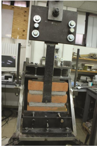
Fig. 1 - Test pattern setup for the single shear test.
