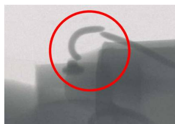
Fig. 14 X-ray inspection point out the wire's break.
